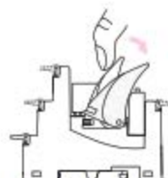
Removing the relay from the socket with a retractor / retractor clip
